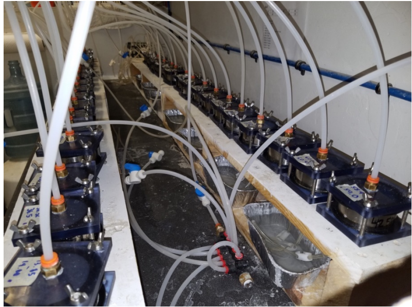
Figure 4. Simultaneous testing of forty cells
