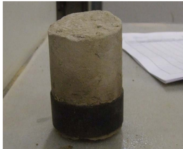
Figure 2. HQ core and test ring
